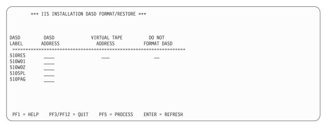
Figure 3. Installation DASD Format and Restore Panel (3390 Model Layout)
